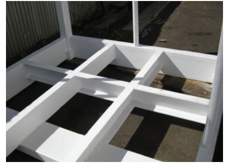
OFFSHORE PIPERACK PANEL SKID
