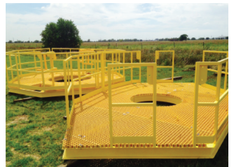
BOP SCAFFOLDING PLATFORMS
